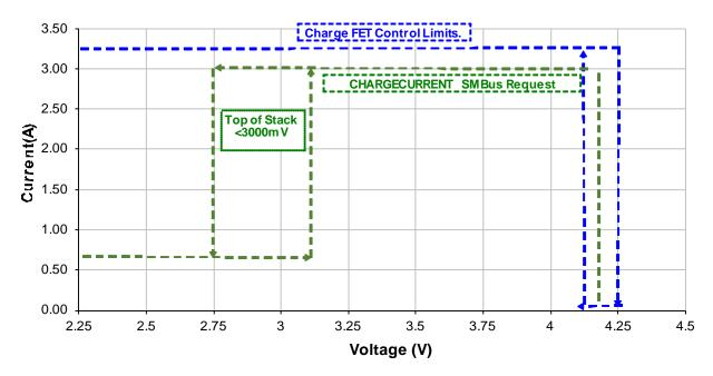
NOTE: The charging current requested from 3.0 to 4.2 V is defined by the temperature of the pack as shown in the preceding charge operating limits graph in this section. A 3.0A charge current is shown in this graph to represent the current defined by said graph.
