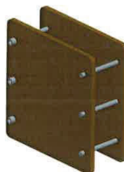
Fig. 2 Diagram of the clamp covered with insulation film 图 2 电池夹具包绝缘膜图
