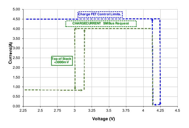
NOTE: The charging current requested from 3.0 to 4.2 V is defined by the temperature of the pack as shown in the preceding charge operating limits graph in this section. A 4.0A charge current is shown in this graph to represent the current defined by said graph.
