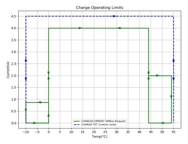
NOTE: If not charging & temperature  $>45^{\circ}C$  then the battery enters Charge-Inhibit where ChargeCurrent() = 0 until temperature  $\leq 44^{\circ}C$ .
