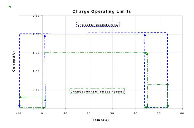
NOTE: If not charging & temperature > 45C then the battery enters Charge-Inhibit where ChargingCurrent() = 0 until temperature <= 44C.
