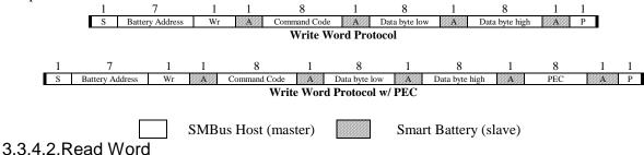
Reading data is slightly more complex than writing data. First the host must write a command to the slave device. Then it must follow that command with a repeated start condition to denote a read from that device's address. The slave then returns two bytes of data.
